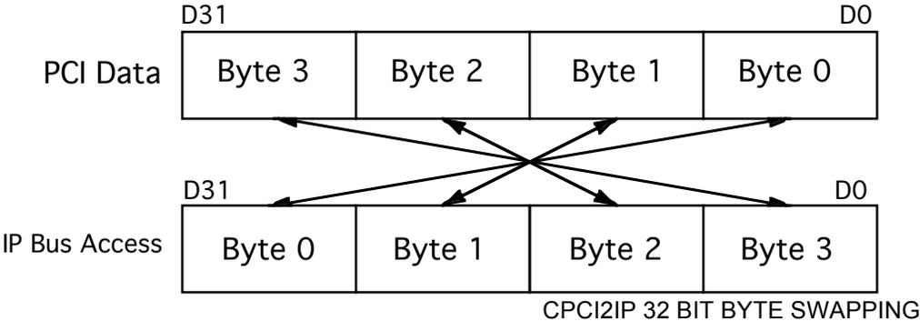
FIGURE 8 CPCI2IP 32 BIT BYTE SWAPPING
