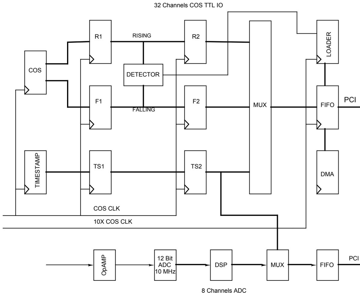
**Figure 2 ccPMC-PARALLEL-TTL-BA18 Operational Block Diagram**
