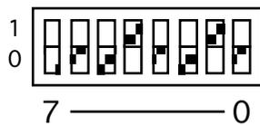
The Design ID and Revision are defined by a 16 bit field allowing for 256 designs and 256 revisions of each. The BA18 design is 0x02 the current revision is 0x03.
