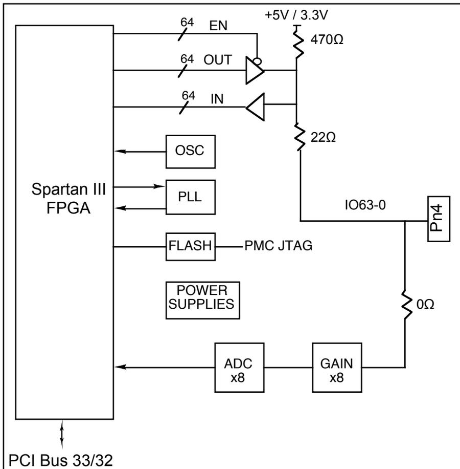
Figure 1 ccPMC-PARALLEL-TTL Block Diagram
