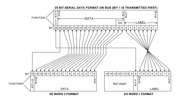
FIGURE 4. MAPPING OF SERIAL DATA TO/FROM WORD 1 AND WORD 2 - 25-BIT FORMAT
